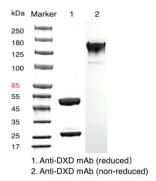
**Anti-DXD mouse mAb** on SDS-PAGE under reduced condition. The purity is 98.2%; **Anti-DXD mouse mAb** on SDS-PAGE under non-reduced condition. The purity is 98.4%.
