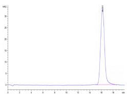
The purity of Biotinylated Human B7-H3 is greater than 95% as determined by SEC-HPLC.
